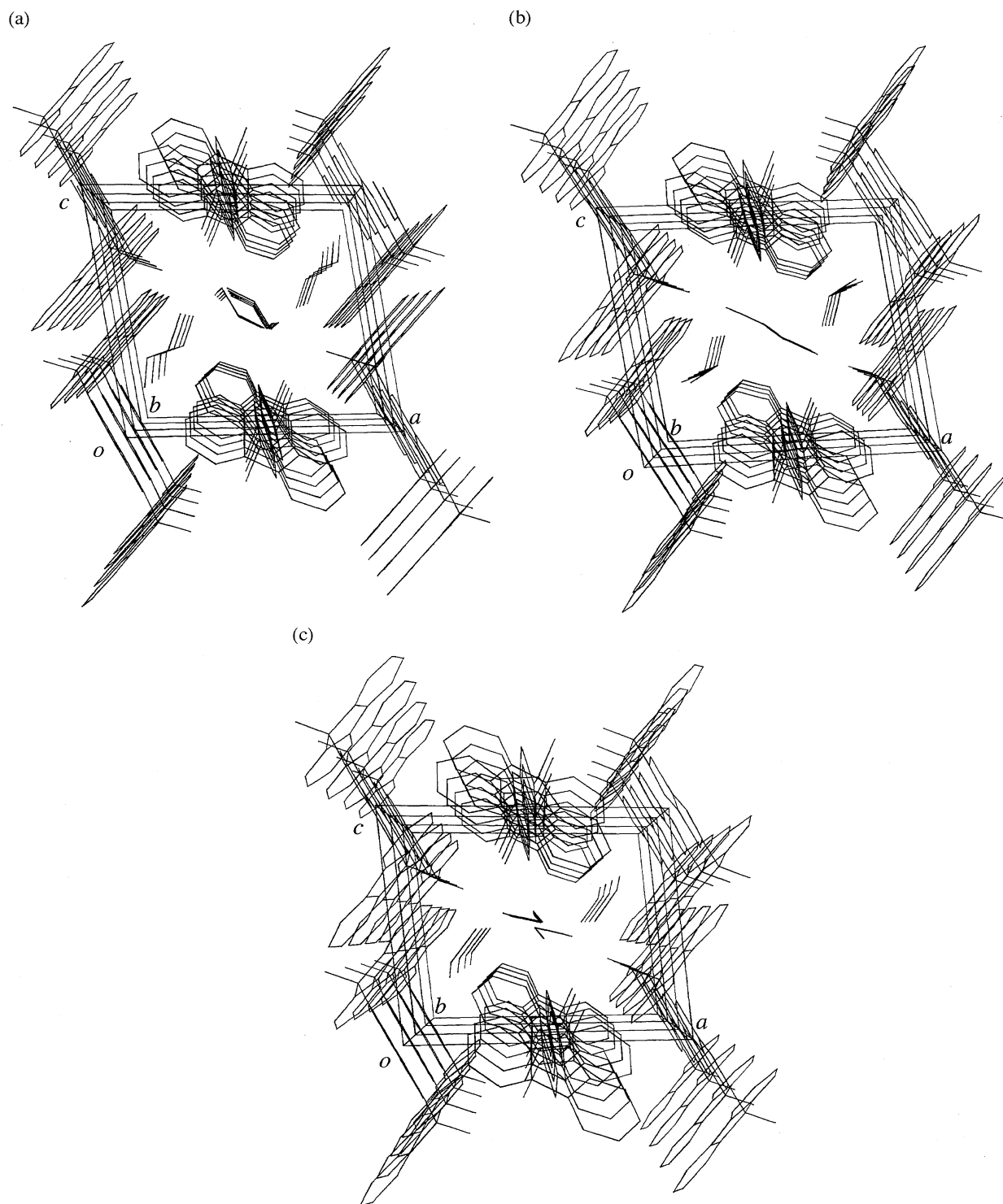
Fig. 1. Crystal structure showing the isostructural inclusion channel viewed along the b axis for three clathrate crystals. a) (\mathbf{1})(n\text{-PrOH})_2 ; b) (\mathbf{1})(i\text{-PrOH})_2 ; c) \beta\text{-(}\mathbf{1}\text{)(EtOH)}_2 . 13)
